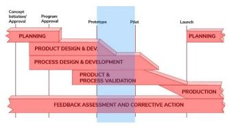
APQP Phase 3 verifies the manufacturing capability and measurement methods.
